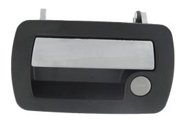
This flush mounted paddle is a redesign of our 030-0450 paddle handle for compartment doors and entrance doors on recreational and specialty vehicles. Containing the same proven mechanical details as previous with a modernized look, it can be used in FMVSS 206 (ECE R11) applications, is power lockable and features two point remote pivot plate and lock cam actuation.
